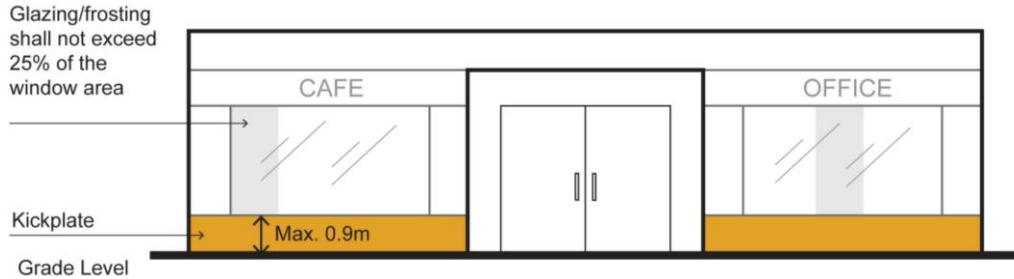
Figure 28. Building Facades Regulations
